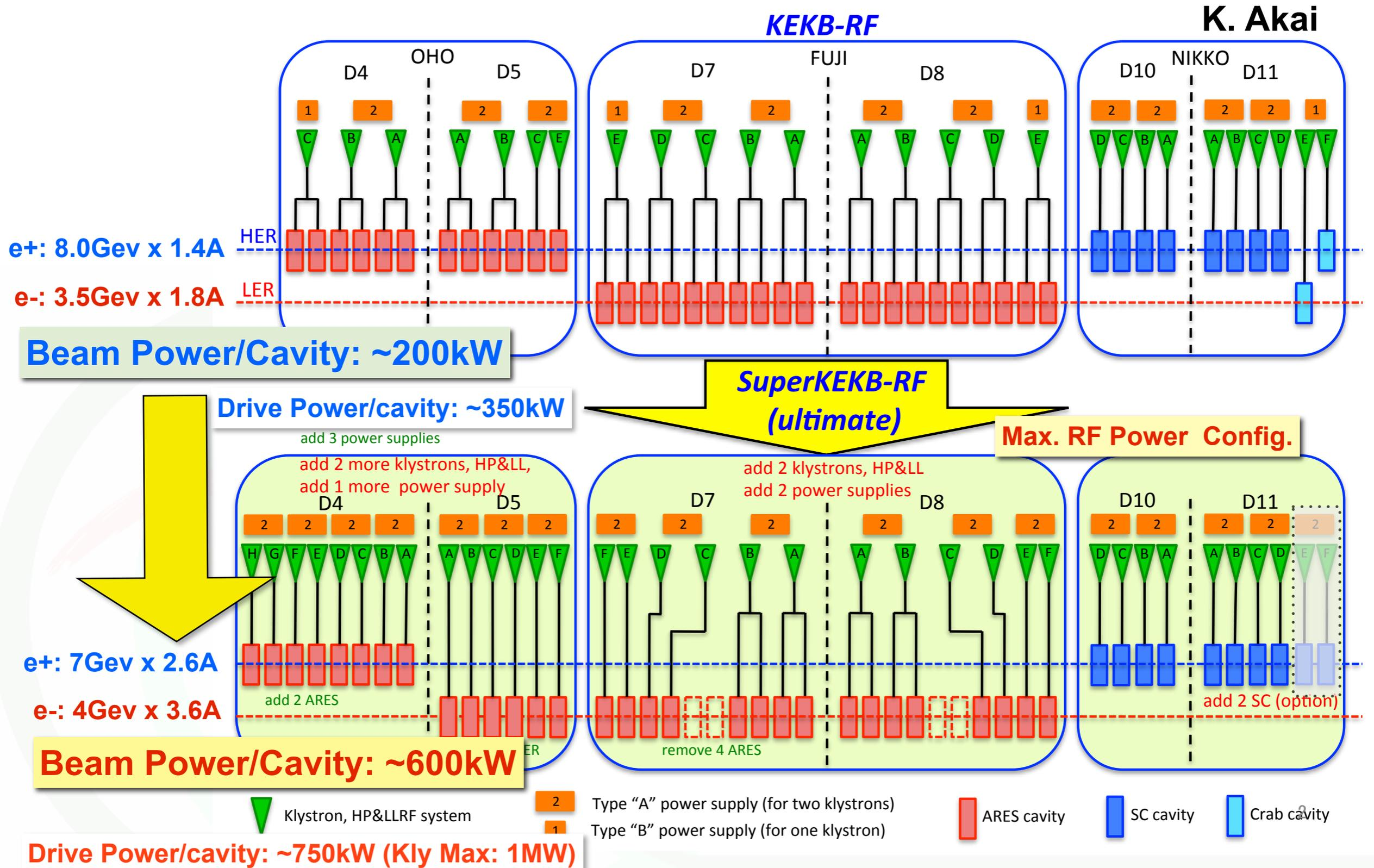
➔ **One-to-one configuration** for every ARES (One klystron drives one cavity unit).
