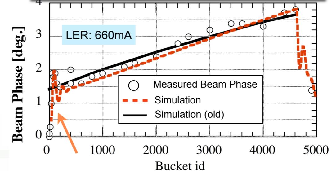
With including the three-cavity structure of ARES in the calculation, the rapid phase change at the leading part of the bunch train can be reproduced by the simulation. It was clarified that the rapid phase change is attributed to the parasitic (0&pi) mode of ARES.
