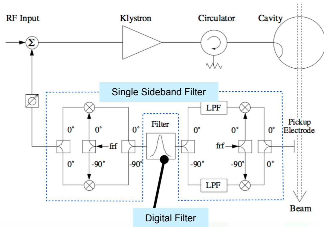
The  $\mu=-1$  mode digital feedback selectively reduces impedance at the driving frequency.
