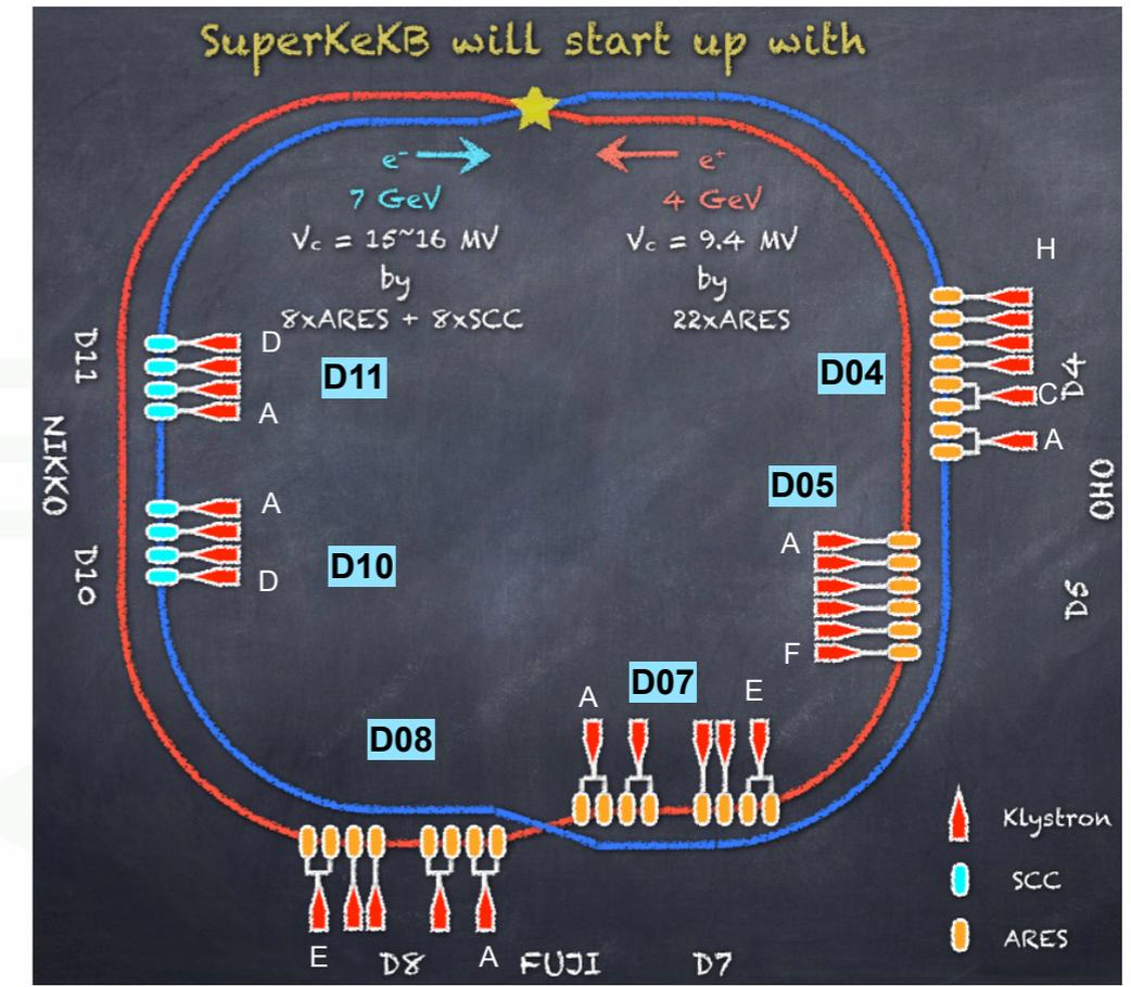
In the several stations (D5A,D5B, D7D, D8D, D10A), the cavities are powered-off and detuned to put out of operation for some reasons.
