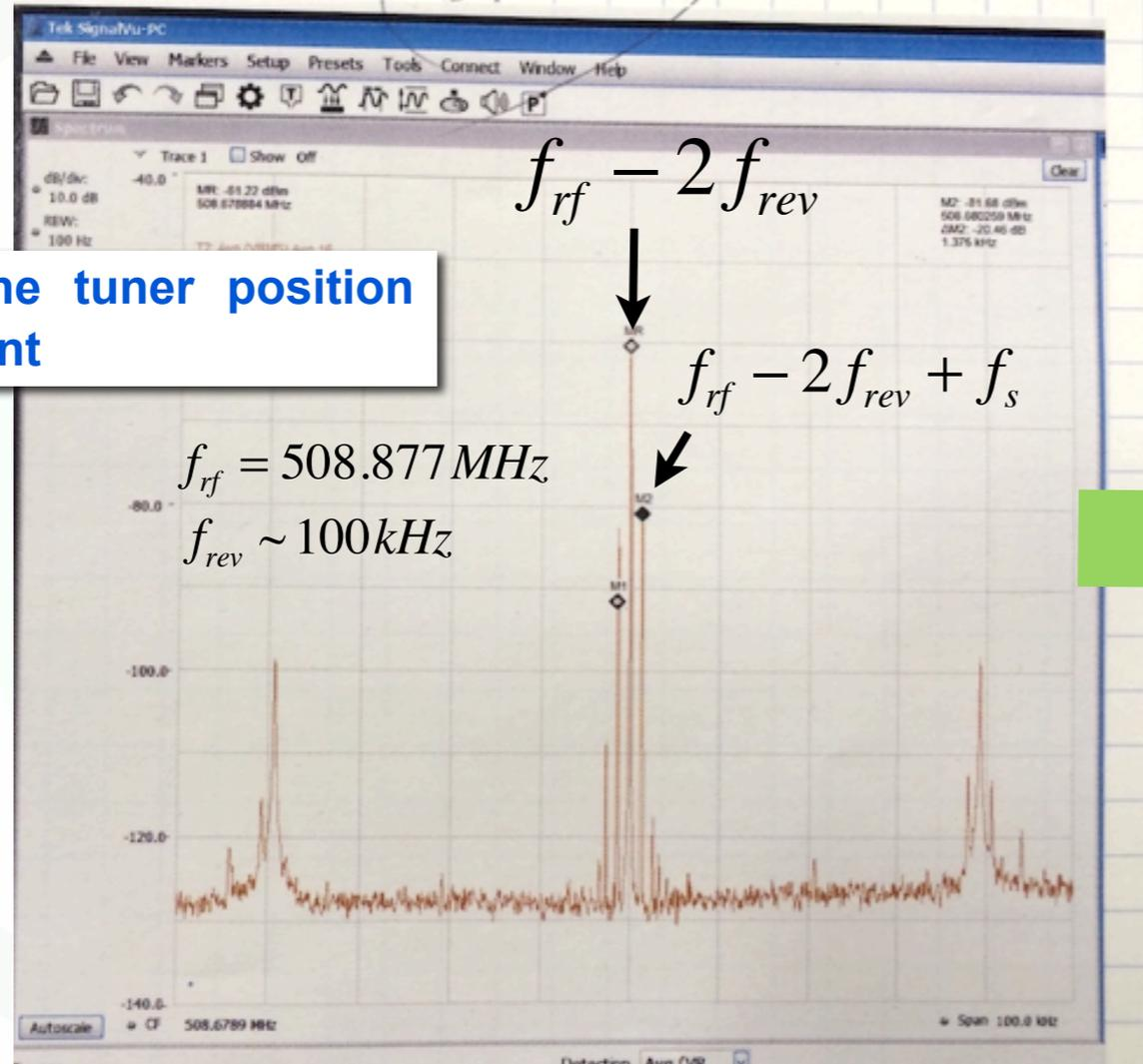
After the tuner position adjustment
