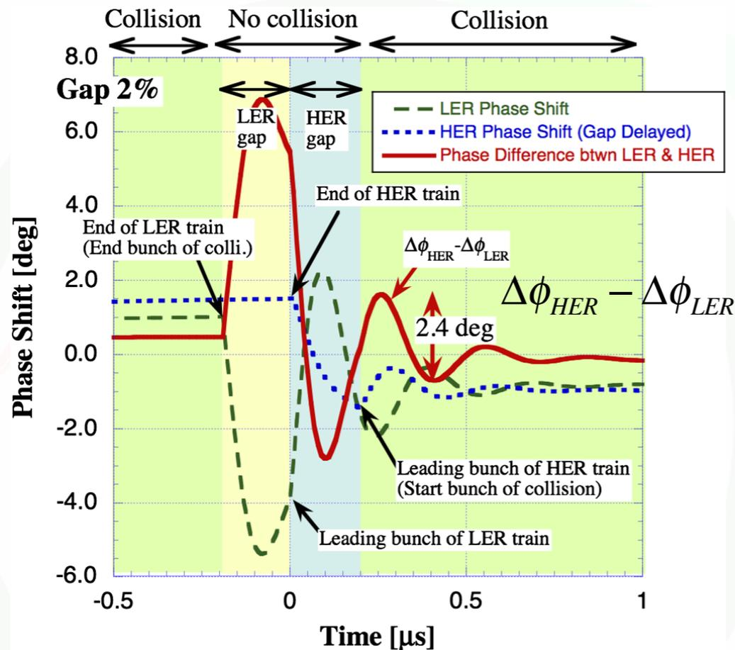
In this case, the collision avoids the largest rapid phase change at the LER leading bunches. Then, the phase difference for the collision is reduced to 2.4 degrees from 5.5 for the collision. However, colliding bunches is reduced to 4% bunch gap equivalent.
