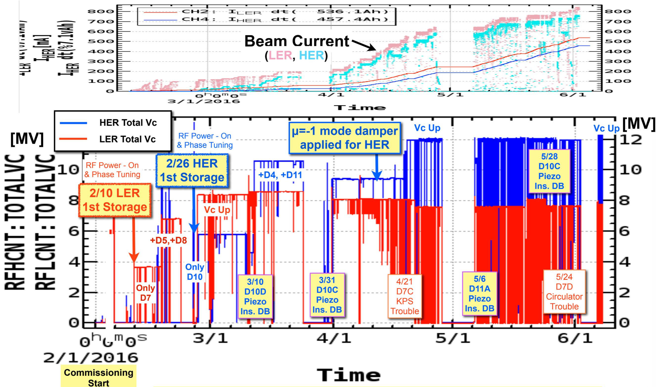
RF system has been providing sufficient acc. voltage without critical trouble.
