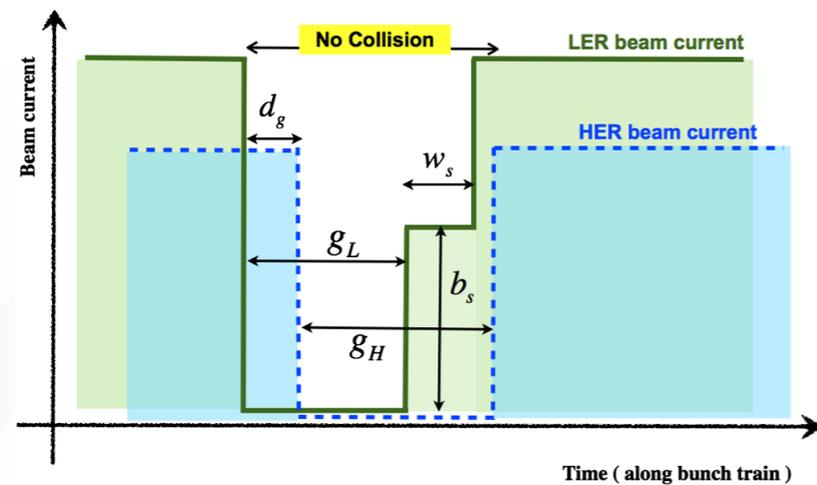
Then, the HER gap delay and the time interval of the first step ( $w_s$ ) are parameters to be optimized.
