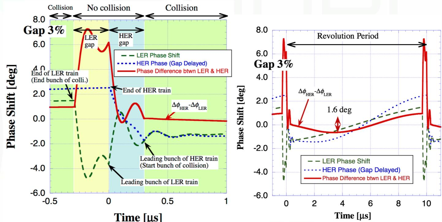
In this case, the phase difference between the two beams almost cancels at the leading part of the train. However, the phase difference along the entire bunch train in the revolution period is increased to 1.6 degrees from the no-delay case.
