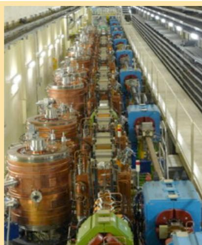
Basically, KEKB RF systems are reused with reinforcement for SuperKEKB.
