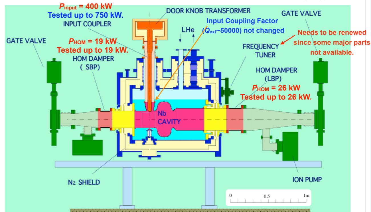
$V_c = 1.5 \text{ MV}$ ,  $P_{\text{beam}} = 400 \text{ kW /cavity}$
