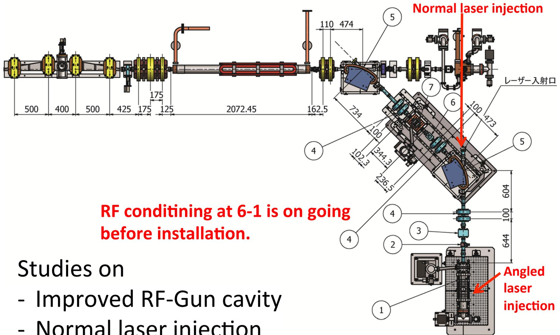
**RF conditioning at 6-1 is on going before installation.**
