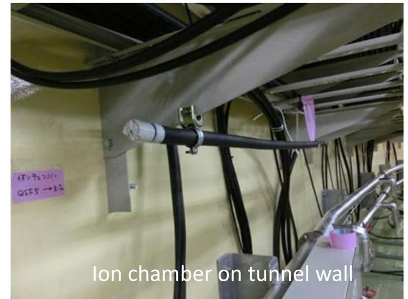
Ion chamber on tunnel wall
