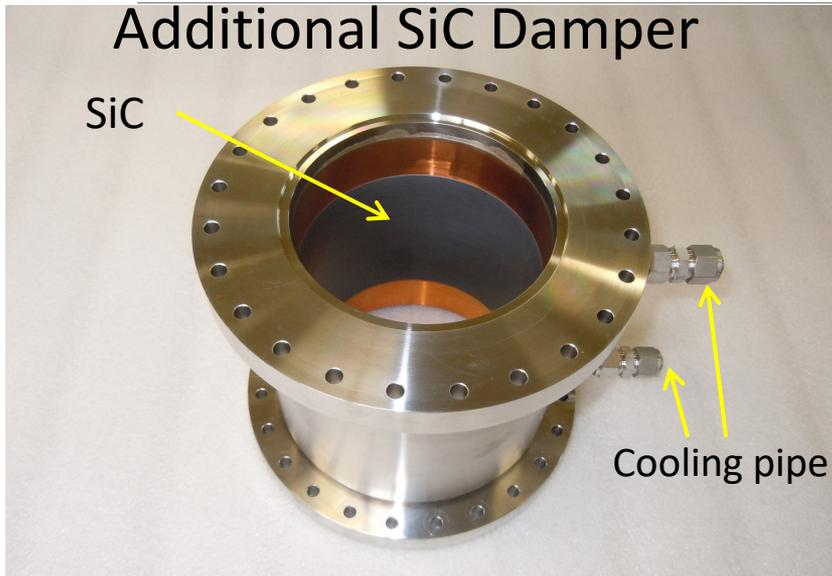
SiC damper can be installed outside of GV of cavity module. There are no risks due to disassembling of cavity module.
