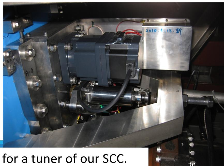
Piezo Stroke : 80  $\mu\text{m}$  in 1000 V
