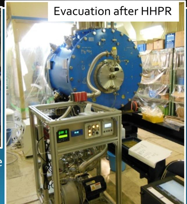
Cavity was dried up by evacuation before setting the coupler and HOM dampers.
