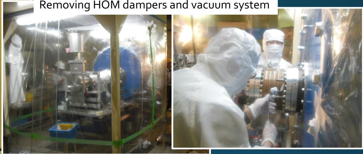
Removing HOM dampers and vacuum system
