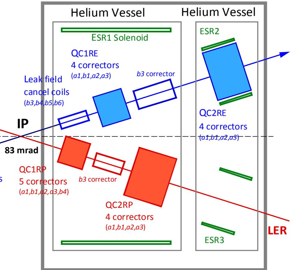
4 SC main quadrupole magnets: 1 collared magnet, 3 yoked magnets
