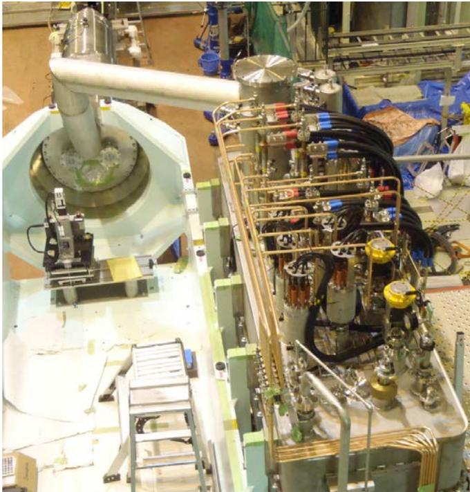
Top surface of the QCSR service cryostat (30 pairs + 1 current leads)
