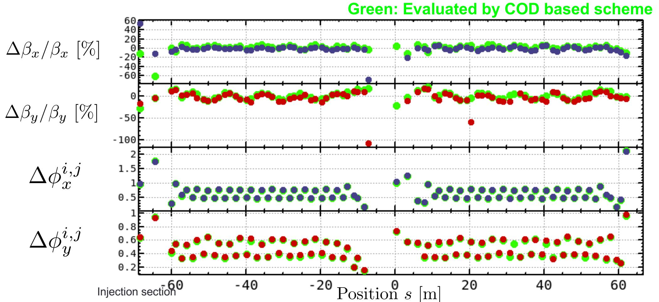
$$(\Delta\beta_x/\beta_x)_{\text{rms}} \sim 11 \% \quad (\Delta\beta_y/\beta_y)_{\text{rms}} \sim 16 \%$$
