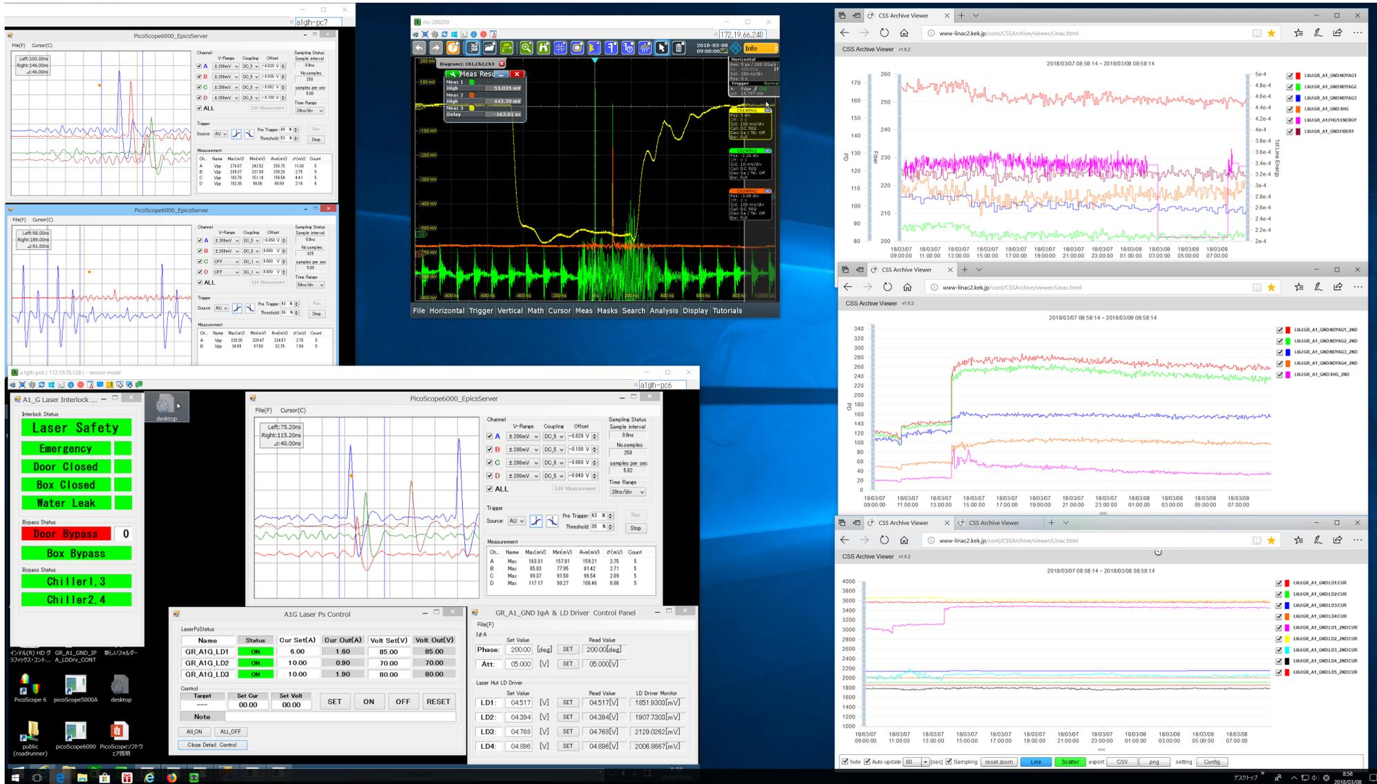
Laser monitors for fiber laser part and every amplifier stage were installed. We can justify the error part immediately from these logs. (SuperKEKB ARC R71)
