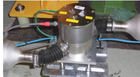
HLS sensor by BINP (Hydrostatic water Leveling System)
