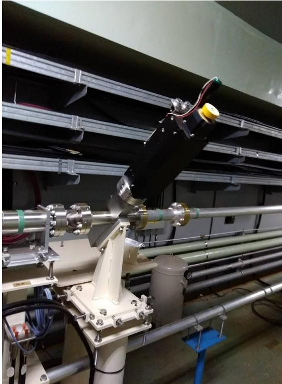
Wire scanner is tilted by 45 degrees from a horizontal plane
