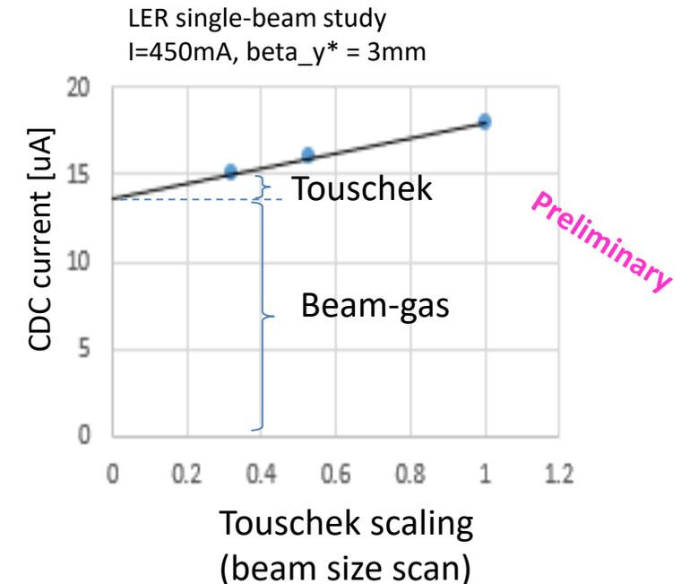
At the end of June, we moved to  $\beta_{y^*}=2\text{mm}$  optics. When  $L\sim 1.2\cdot 10^{34}$  is achieved with 800mA, **BG was three times too high to turn on Belle2.**
