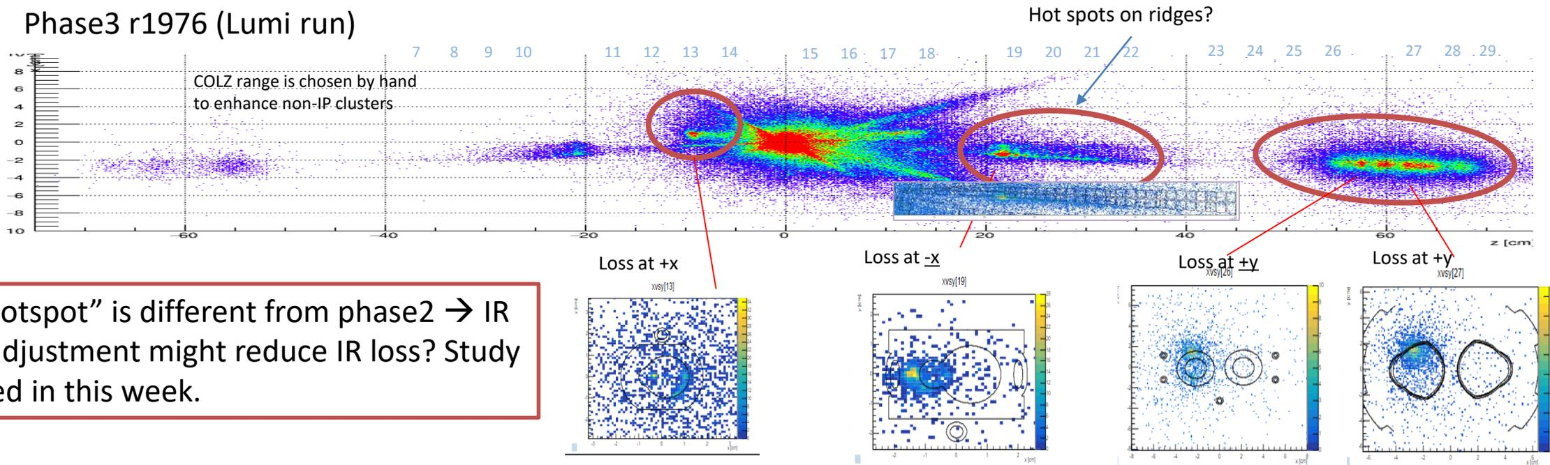
LER “hotspot” is different from phase2 → IR orbit adjustment might reduce IR loss? Study planned in this week.
