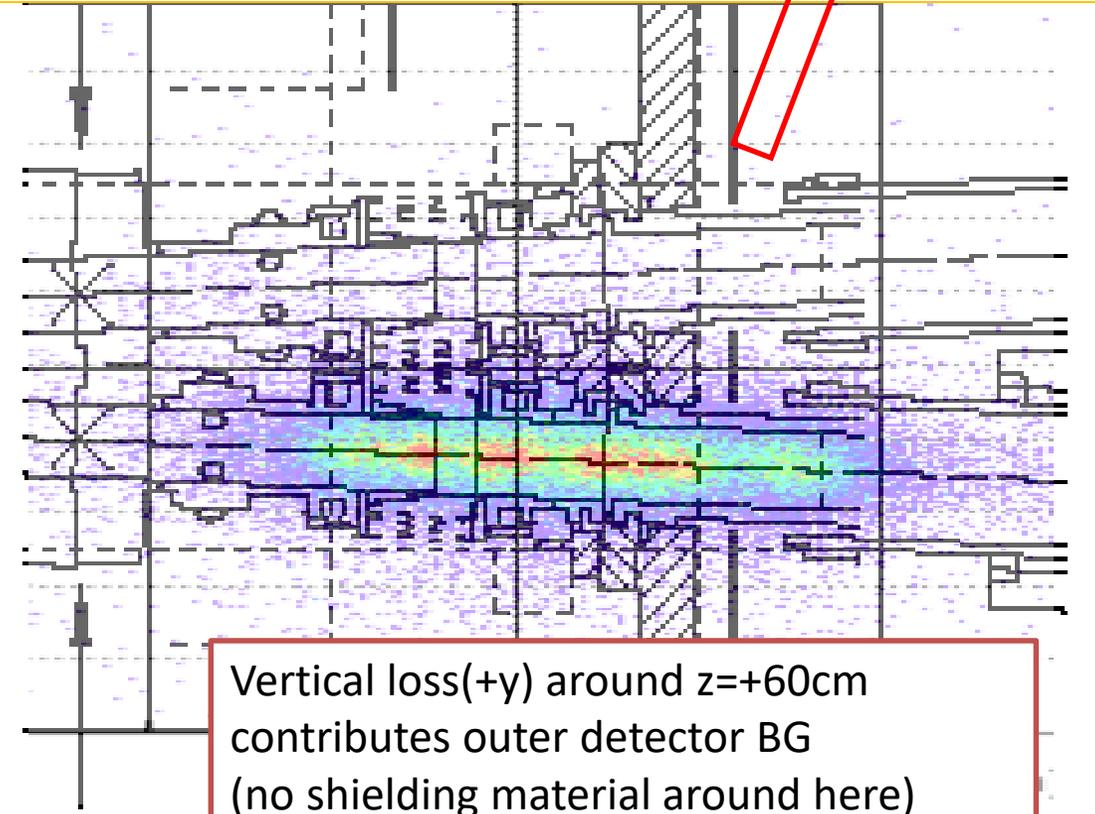
Vertical loss(+y) around  $z=+60\text{cm}$  contributes outer detector BG (no shielding material around here)
