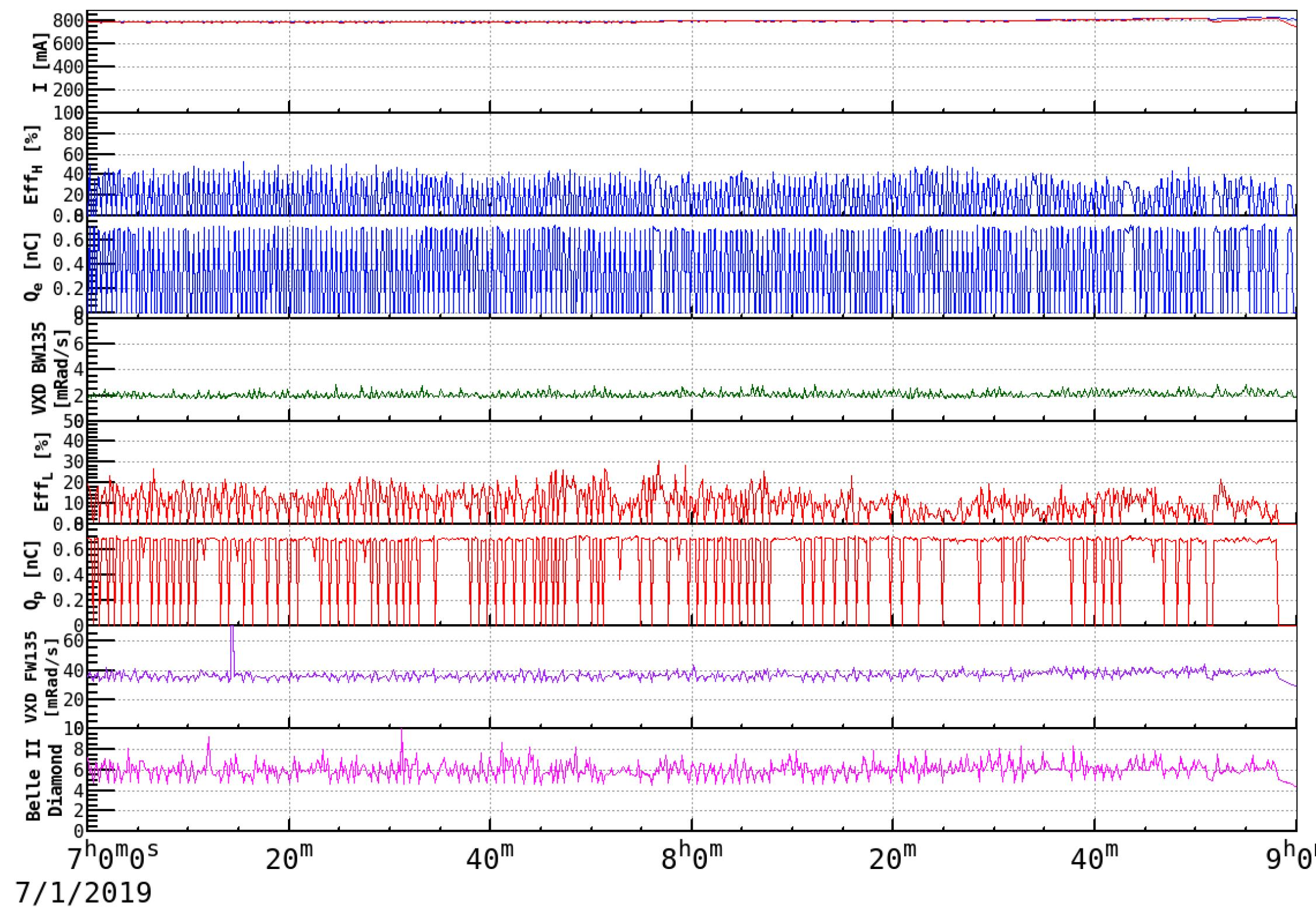
The injector capability limits the max. beam current in LER.
