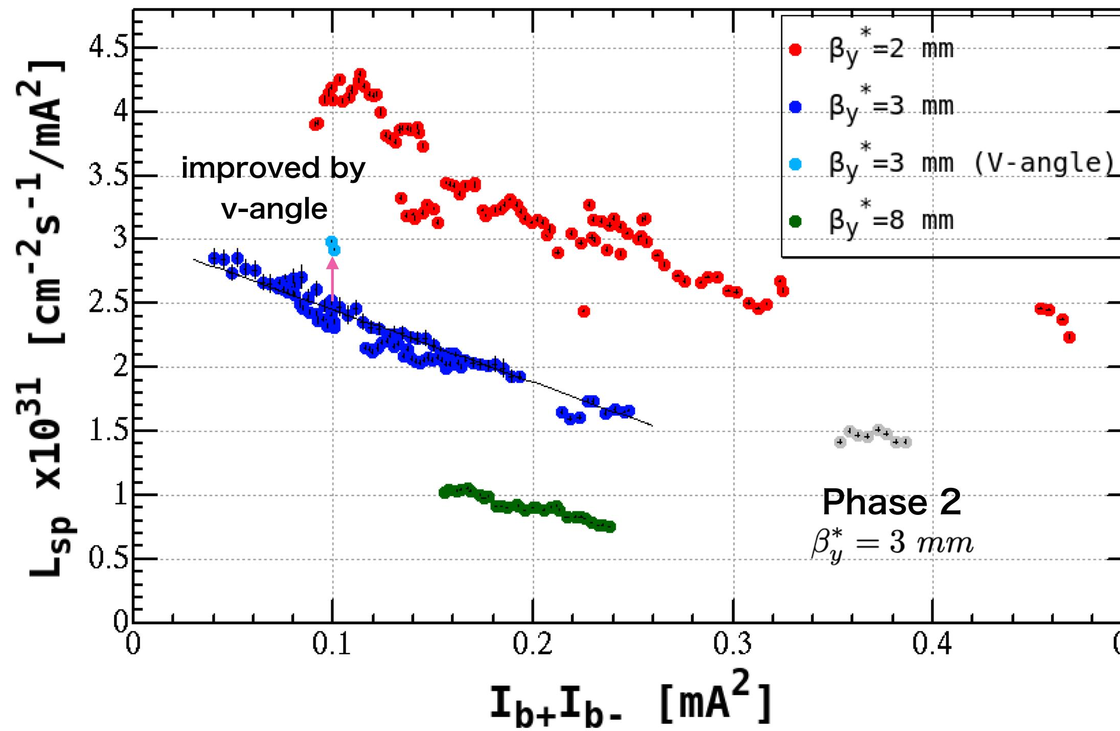
The specific luminosity is improved by squeezing the vertical beta function at IP.
