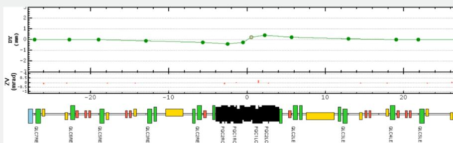
The large vertical dispersion leaked from IR was not correctable owing to hardware limit of correctors.
