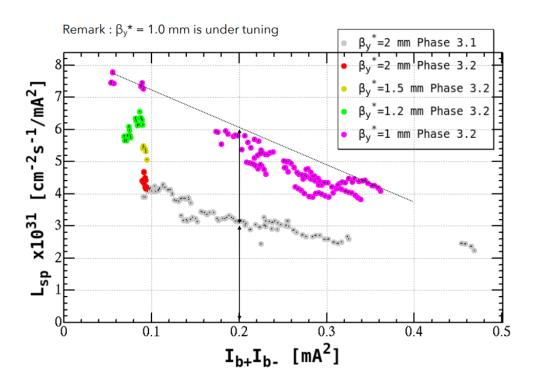
$\beta_y^*$  is squeezed to 1mm in 2019. Specific luminosity is lower than expected value (~9x10<sup>31</sup>)at even low current. The beam-beam parameter is limited at 0.02 (HER is lower, due to LER blowup).
