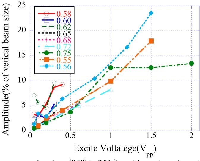
Larger response from tune (0.58) to 0.63 (tune + beam-beam tune shift)
