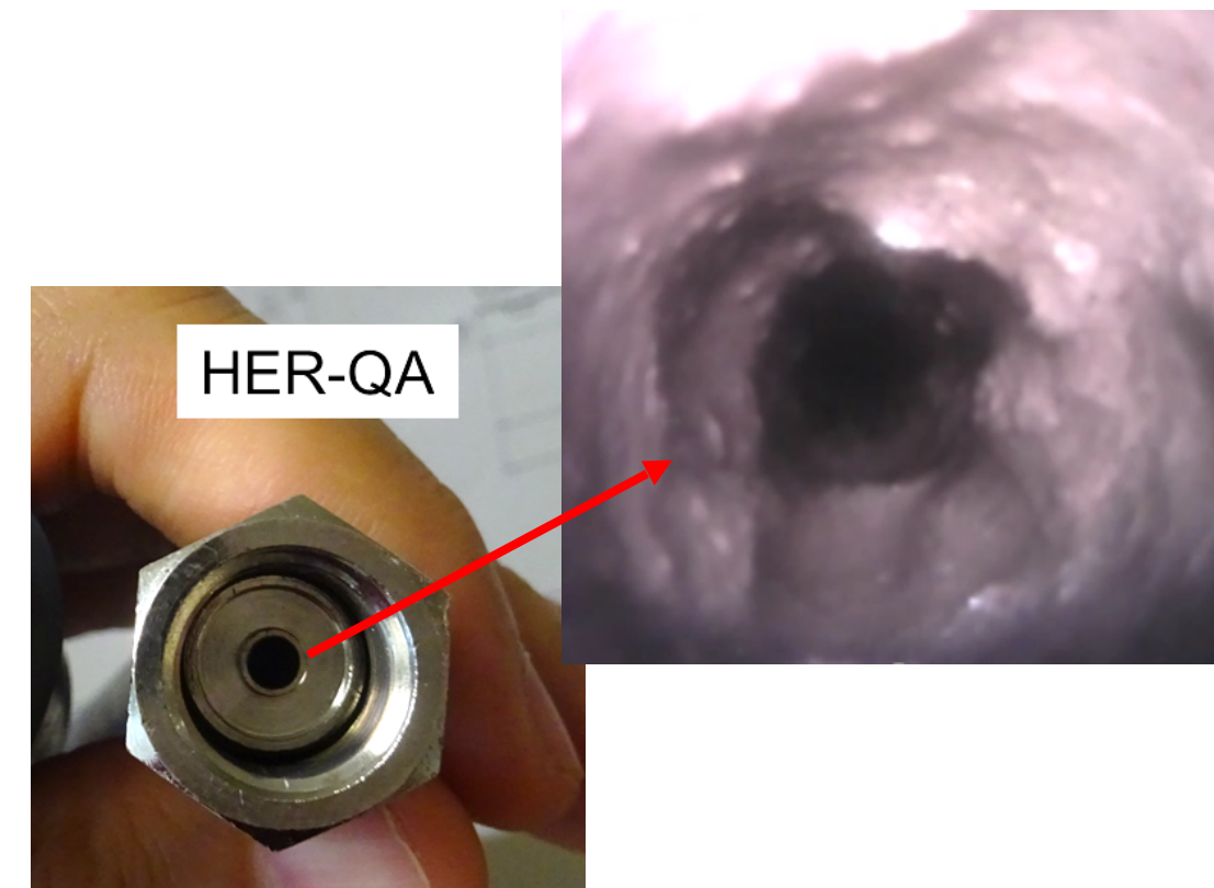
Entrance of water hose of a magnet
