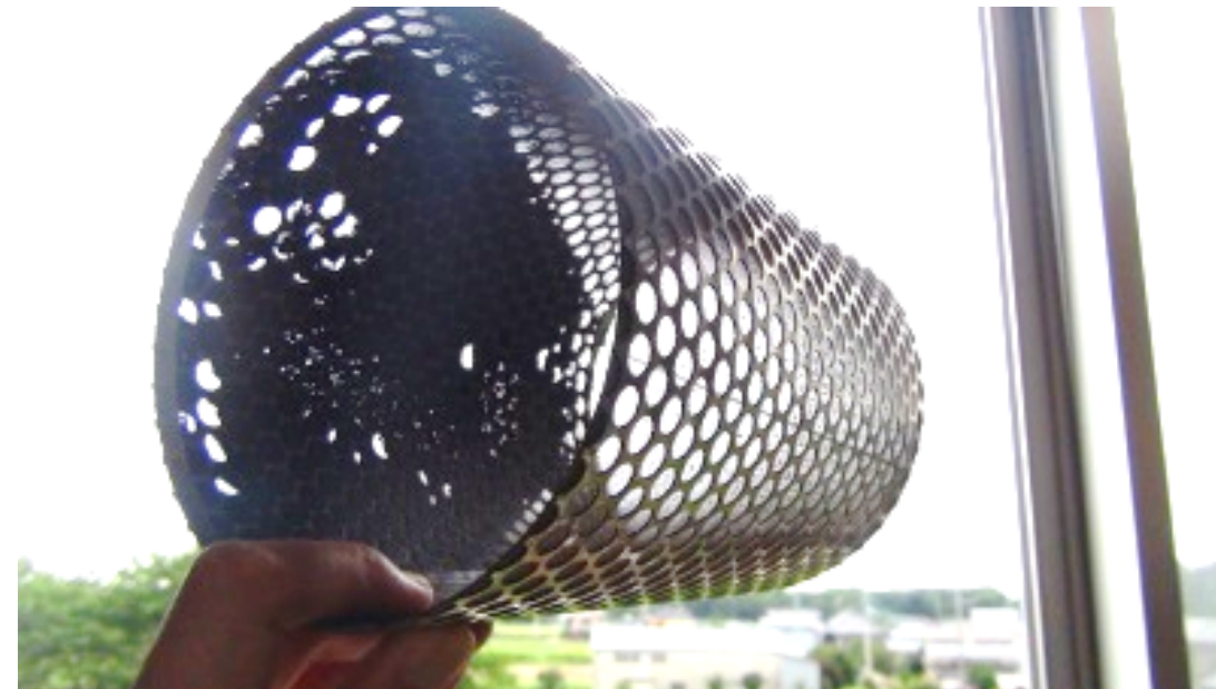
A strainer just before a pump
