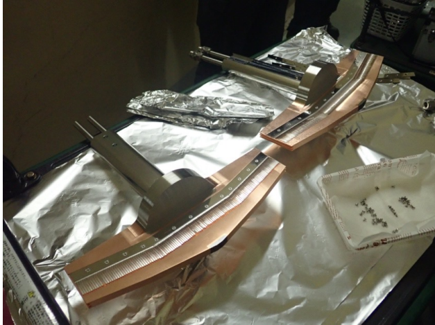
Attach RF-fingers to the spare jaws.
