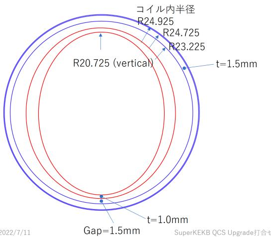
1. Increase QC1P aperture (vertical) from 13mm to (18mm) 20.7 mm
