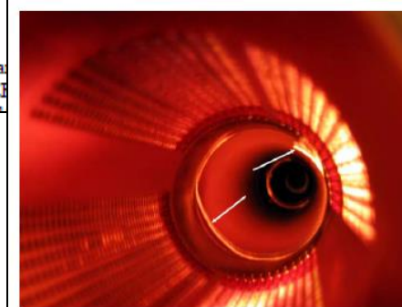
Figure 9: Dislocated rf seal in the LER vacuum chamber.
