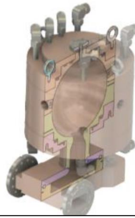
New pulse compressor Spherical-Cavity Pulse Compressor (SCPC)
