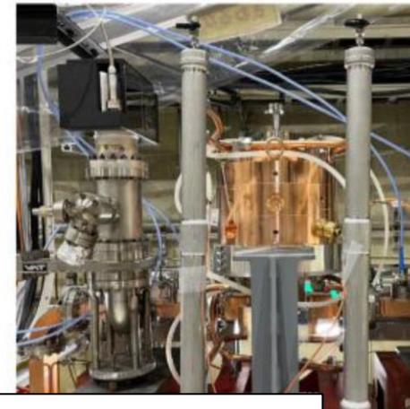
New pulse compressor Spherical-Cavity Pulse Compressor (SCPC)
