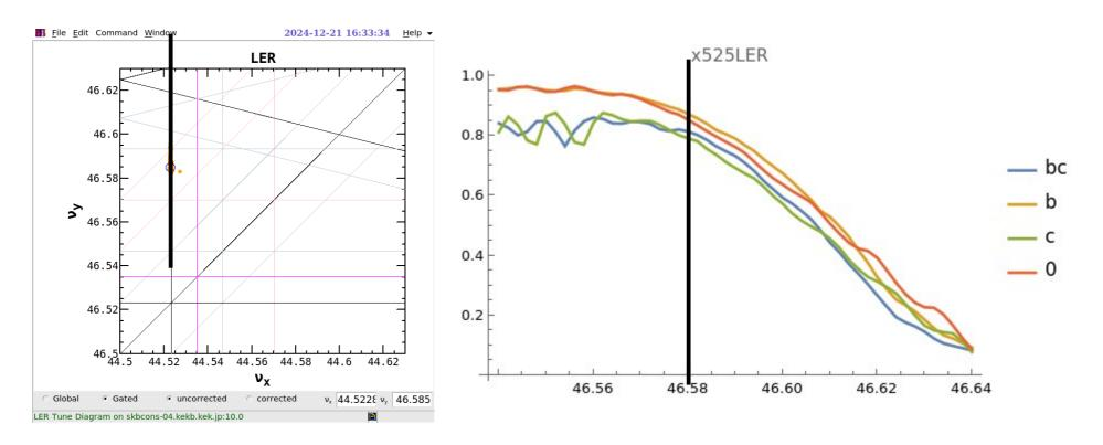
Chromatic coupling resonance ~ 0.575. Lower injection eff with higher tune.
