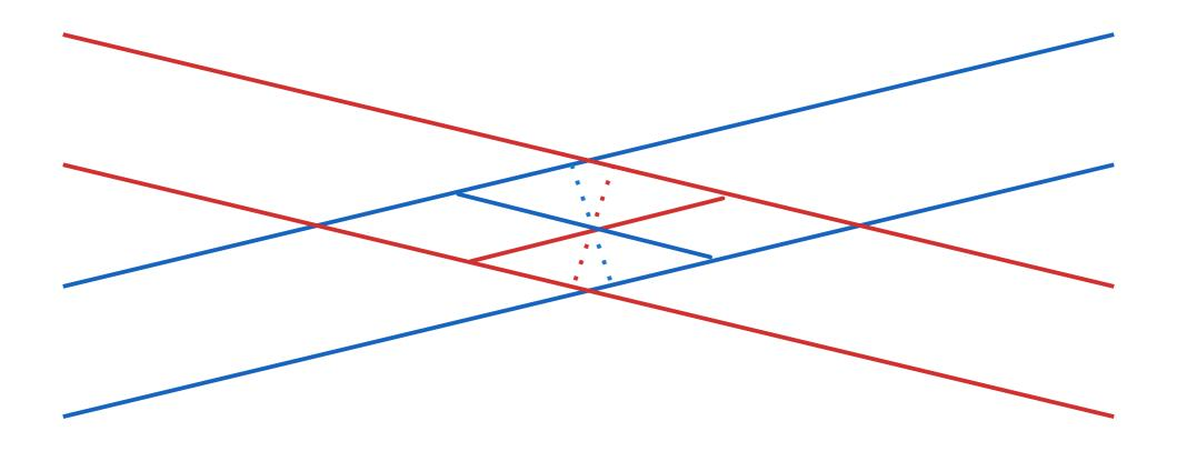
Lsp is increased with more low beta crossing. Extra beam-beam effect is also reduced.
