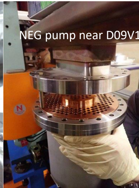
D09V1 Head Color of Cu coating changed SR? HOMs?
